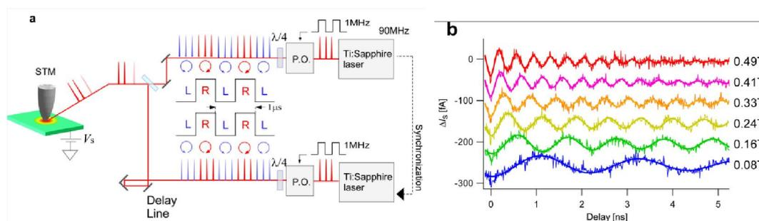
**Fig.1.** (a) The schematic of the OPP-STM. (b) The magnetic field dependence of spin precessions on GaAs(110) under the OPP-STM setup, the spin precession occurs at the Larmor frequency  $\omega = g\mu_B B / \hbar$ , where  $g$  is the Landé's  $g$  factor,  $B$  is the magnetic field,  $\mu_B$  is Bohr magneton and  $\hbar$  is Dirac constant.
